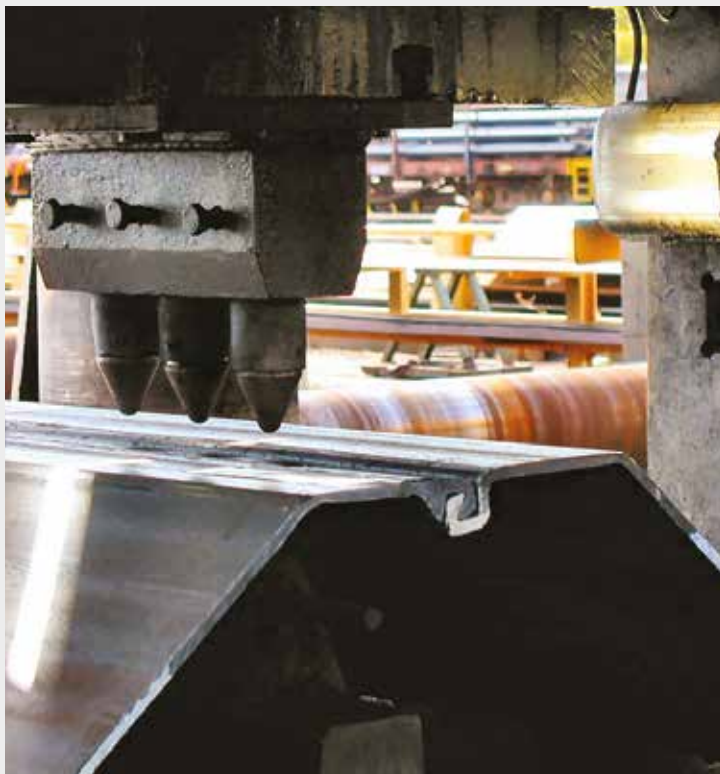
Fig. 8. Special crimping pattern for AZ infill sheet piles and crimping at the rolling mill.
