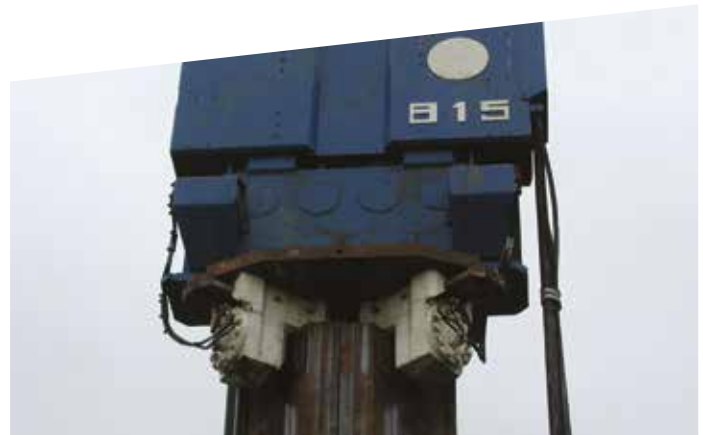
Fig. 13. Double clamps for a vibratory hammer.
